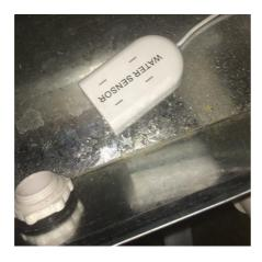
If moisture is sensed the alarm will sound. This is an audible cue for a potential drainage fault and is in addition to the safety drain installed into your eave. Your eave drain would normally be dripping if the alarm is sounding.
